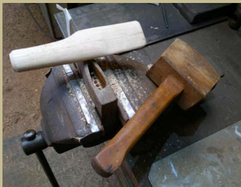
5. Driving out the handle stub with a bit of smaller axe shaft as a drift.
