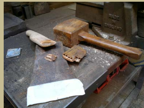
6. Axe eye cleared out, ready to re-handle.
