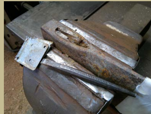
3. Cold chisel to remove metal wedges, in this case a bit of joist
